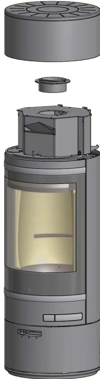
Mount the ceramic gasket on the connecting piece
