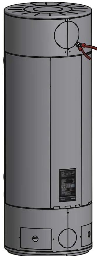
Tilt the wire-cutter downwards and the cover plate will loosen.
