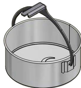
In order to put back the ash container in the stove, place the guide mounting in the positioning hole. Turn the ash container so that the handle is in the closed position.
