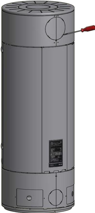
Tilt the screwdriver downwards and the cover plate will loosen.
