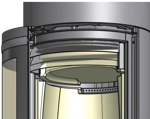
Turn the baffle plate 90°, and lower it out through the combustion chamber.
