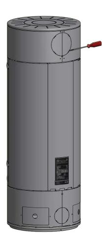
Tilt the screwdriver downwards and the cover plate will loosen.
