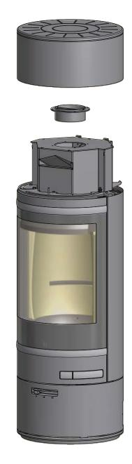
Mount the ceramic gasket on the connecting piece
