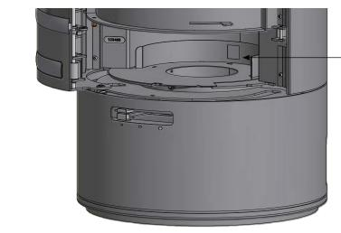
Positioning hole for guide mounting on ash container
