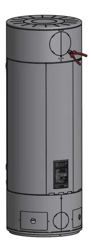
Tilt the wire-cutter downwards and the cover plate will loosen.
